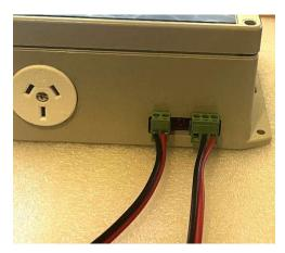
The reason for the two size connectors is to avoid the incorrect sensor being plugged into the wrong position. The 3 pin connector is the roof sensor and the 2 pin connector is the pool sensor.
