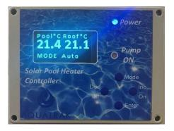
When operated in Manual mode the Off and On buttons will turn the pump off and on. Please note that there is a small de3lay before the pump turns off and on once the button is pressed. This is to ensure the pump is not turned on and off and on too quickly which can cause a current spike and trip a circuit breaker, depending on the type of pump being used.
