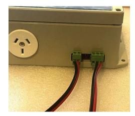
The reason for the two size connectors is to avoid the incorrect sensor being plugged into the wrong position. The 3 pin connector is the roof sensor and the 2 pin connector is the pool sensor. The wires within the plug have no polarity and can be wired up in either terminal.
