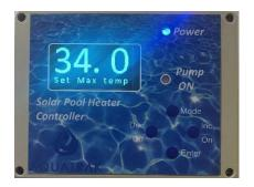
Once the desired temperature is set press the Enter button again. If you do not press the button for 20 seconds than the system will automatically save the current setting and return to the normal menu.
