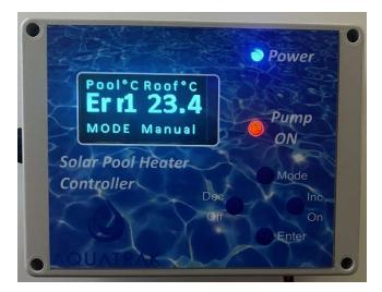
If the controller shows a faulty or erroring sensor check that the plug is plugged into the controller.
